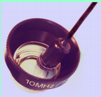
Fig. middle (both): DRG work place. Characteristics of the pulsed Doppler probe in the contact glass: 10 MHz, piezo- \varnothing 4 mm, Doppler sample-volume size variable axially 1-10 mm, laterally fixed at 1 mm (-6dB). The sample volume is automatically placed at a depth of 20-30 mm, according to the length of the eyeball, as recorded by A-mode scan of the same probe. Angle of probe to eye axis = 10° (OBERMAIER). Comprehensive evaluation of the central retinal arteries (CRA) included supplementary CW-Doppler examinations of the extra- and intracranial carotid flow. Fig. left: Transducer with contact glass: Schematic illustration. Fig. right: DRG-graph displaying systolic Doppler-shift of 1 kHz corresponding to a velocity of 7,4 cm/s.
