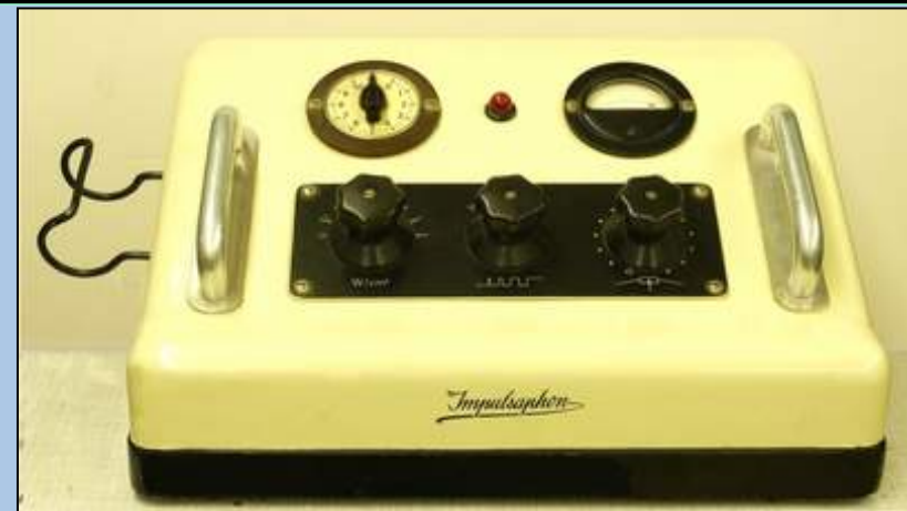
Fig. right: Console: Connecting load 100 VA, time switch, controller W/ cm 2 in 4 steps from 0 - 3 W/cm 2 . Impulse- and continuous operation, controller for switch options (ratio ON/OFF) in 4 steps (1/20, 1/10, 1/5, continuous operation). Tuning controller for the applicator with indicating instrument, control of coupling. Nominal frequency 1000 kHz; max. acoustic power 15 W, emitting surface of the applicator 5 cm 2 , average power density 3W/ cm 2 .
