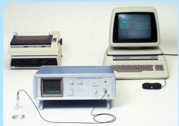
Work station for biometry of the eye with GBS-console (front), A-mode transducer, Commodore V64 computer, printer.
