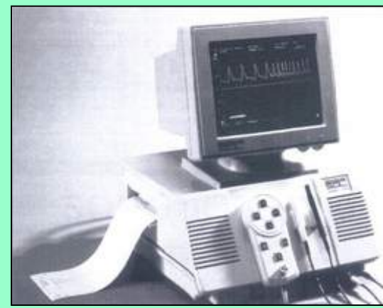
Fig. middle (both): DRG work place. Characteristics of the pulsed Doppler probe in the contact glass: 10 MHz, piezo- \varnothing 4 mm, Doppler sample-volume size variable axially 1-10 mm, laterally fixed at 1 mm (-6dB). The sample volume is automatically placed at a depth of 20-30 mm, according to the length of the eyeball, as recorded by A-mode scan of the same probe. Angle of probe to eye axis = 10° (OBERMAIER). Comprehensive evaluation of the central retinal arteries (CRA) included supplementary CW-Doppler examinations of the extra- and intracranial carotid flow. Fig. left: Transducer with contact glass: Schematic illustration. Fig. right: DRG-graph displaying systolic Doppler-shift of 1 kHz corresponding to a velocity of 7,4 cm/s.
