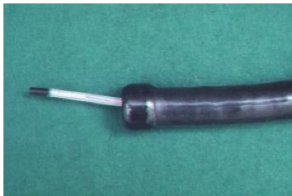
Figure 21 A one-dimensional ultrasound probe (4 MHz) inserted through a commercially available gastroscope (Source: H. Lutz).
